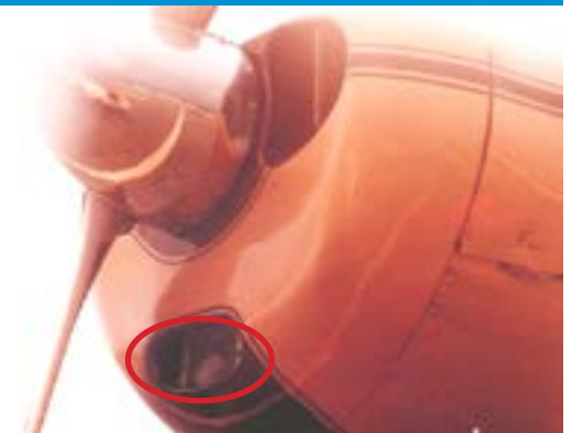
Ice in the airplane's air filter.
