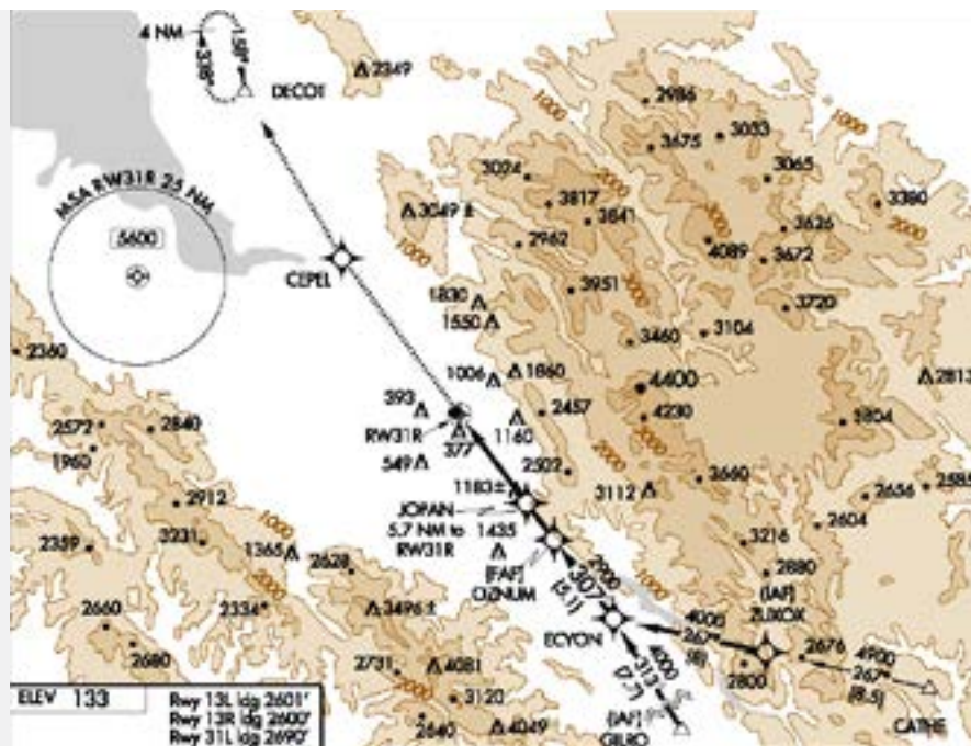
Fig. 8-6. Plan View of the Reid-Hillview GPS RWY 31R approach.
